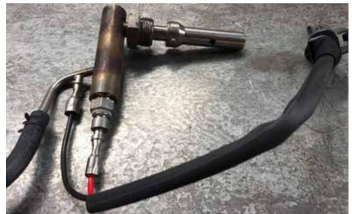
It common for people to mistake an issue with the temperature sensors when a code description like this is displayed- P244C Catalyst temp too low. This temperature sensor in fact is reading correctly and in turn, the correct signal is being sent to the engine computer unit. (ECU). For the DPF to perform a
